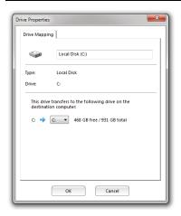
Click on a drive and hit 'Properties' to open the screen for choosing a different drive on the target computer.
