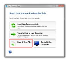
Select *Drag & Drop Files* in the Tools screen to manually transfer files and folders BETWEEN computers.
