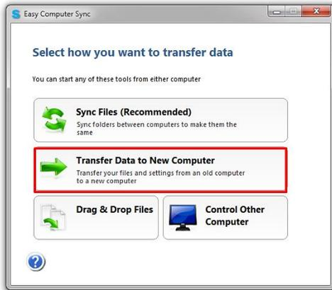
1. Select **Transfer Data to a New Computer** in the Tools screen to migrate data from an old to a new computer.
