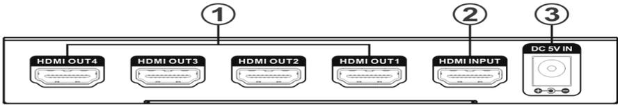
1. HDMI OUT1....4....8: Connect the destination displays to these ports
